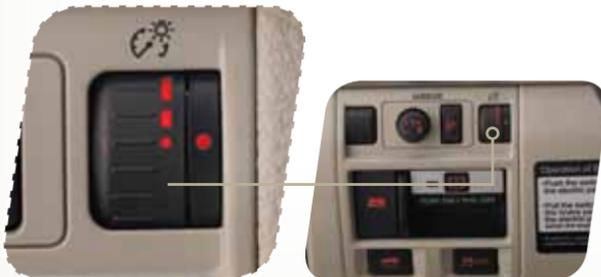
While the light switch is on, rotate the dial downward to dim the instrument panel illumination. Rotate the dial upward to make the illumination brighter. When the dial is fully rotated upward, the instrument panel illumination becomes full bright.
